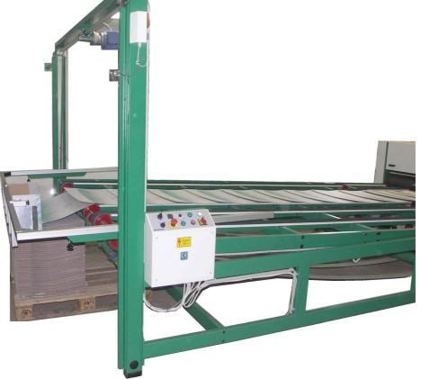
The universal and automatic unloader and stacker device is a kind of supplementary equipment for the packaging and printing machines. It can be fitted to any type of cutting, printing or laminating machine with automatic feeding, even at a later date.
